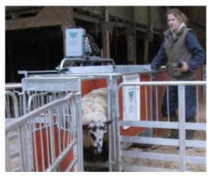
drafting controller to open and close the relevant gates when a tag is read. Sheep can also be drafted by weight by setting up the parameters on the Handheld Stock Recorder.
